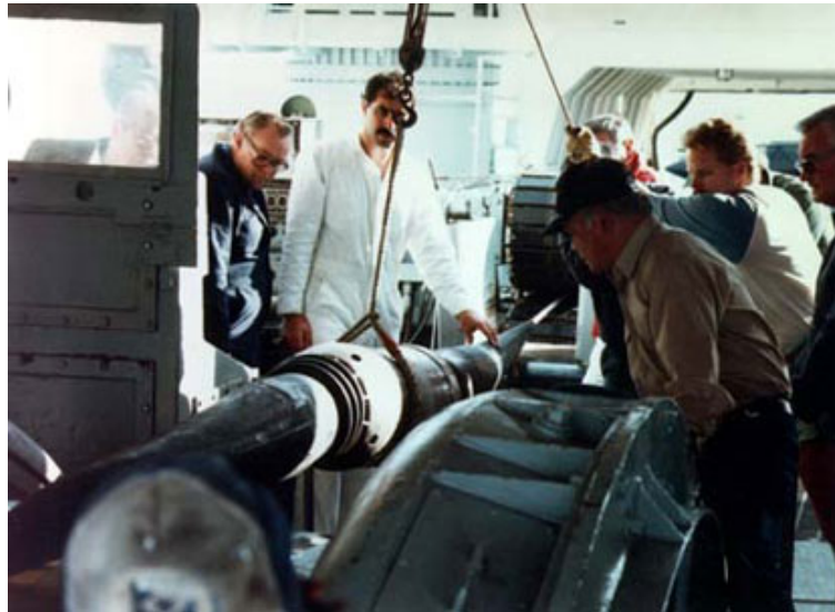
TAT-8 cable and repeater (signal booster) about to pass through the cable laying engine on the deck of the cable ship Long Lines . Image courtesy of AT&T.
