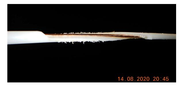
**Figure 2:** Photograph of lightweight cable damage caused by entanglement with a FAD mooring near the Philippines in 4,000m water depth. Note that the polyethylene insulation has been stripped by the FAD mooring exposing the copper conductor.
