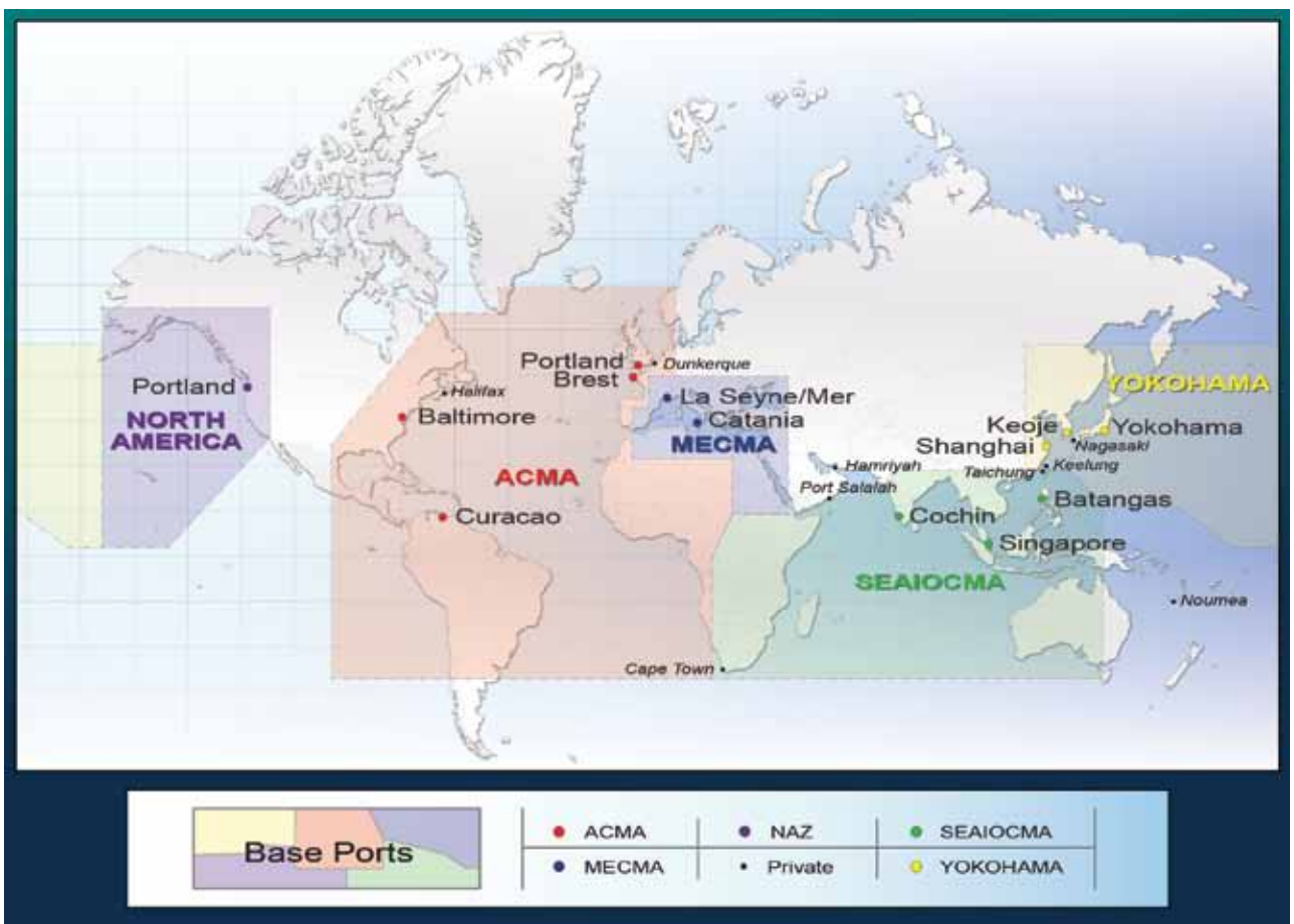
Above, the areas covered by the five “zone” agreements for submarine cable systems as well as the base ports for many of the “private” agreements. At any given time roughly half of the world’s more than 40 cable ships are laying new lines while the other half are either contractually performing maintenance/repair or are on standby.
