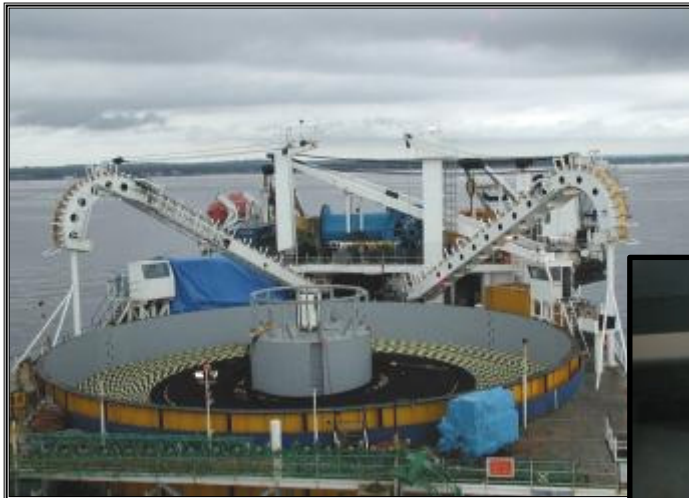
Power cable storage tank on laying ship
