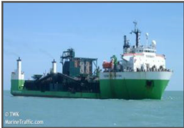
Rock Placement Vessel Source: Marine Traffic
