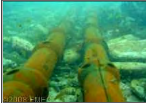
Articulated Pipe Source: EMEC
