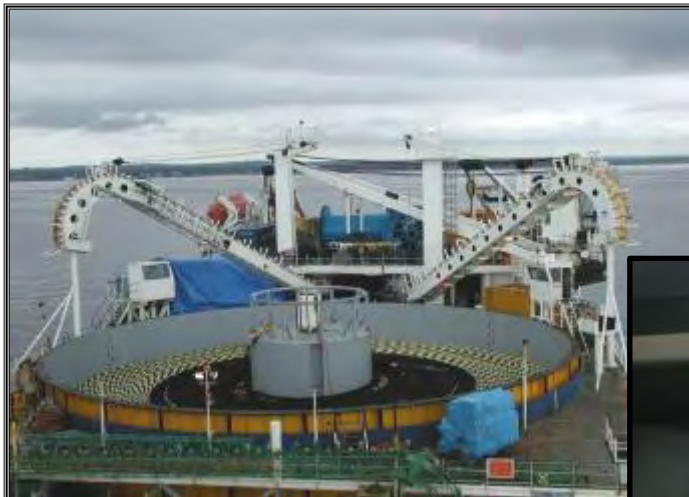
Power cable storage tank on laying ship
