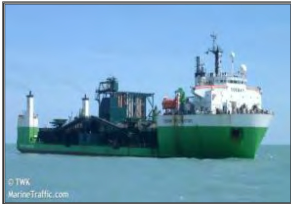
Rock Placement Vessel Source: Marine Traffic
