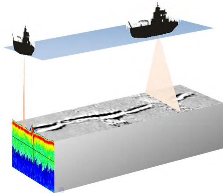
**Plate 8: Schematic image of the combination of SES and SSS measurement**
