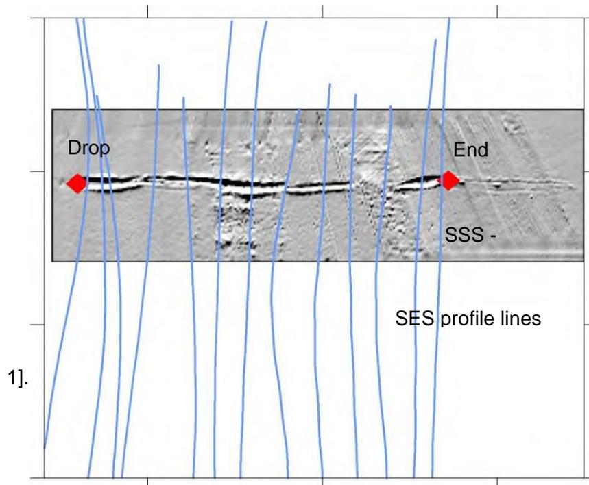
**Plate 9: SES profile lines [blue] and SSS image of an anchor track measurement**
