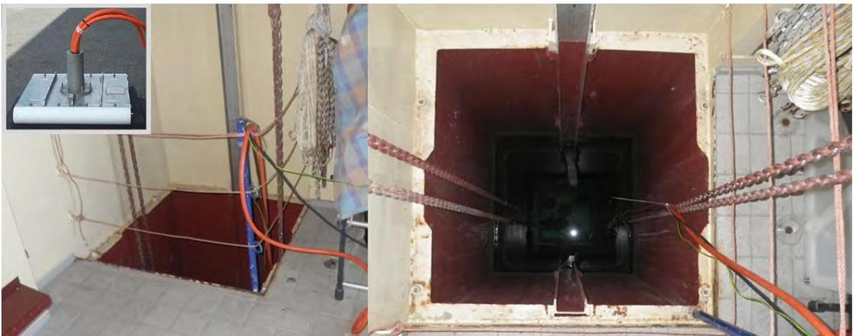
**Plate 2: Hydrographic shaft on VWFS Wega accommodating the SES oscillator**
