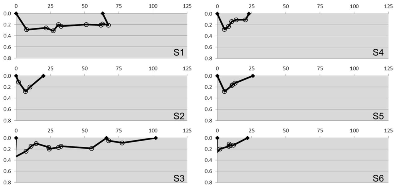
Plate 15: Summary of all anchor tracks [depth profile] in test area BSH South
