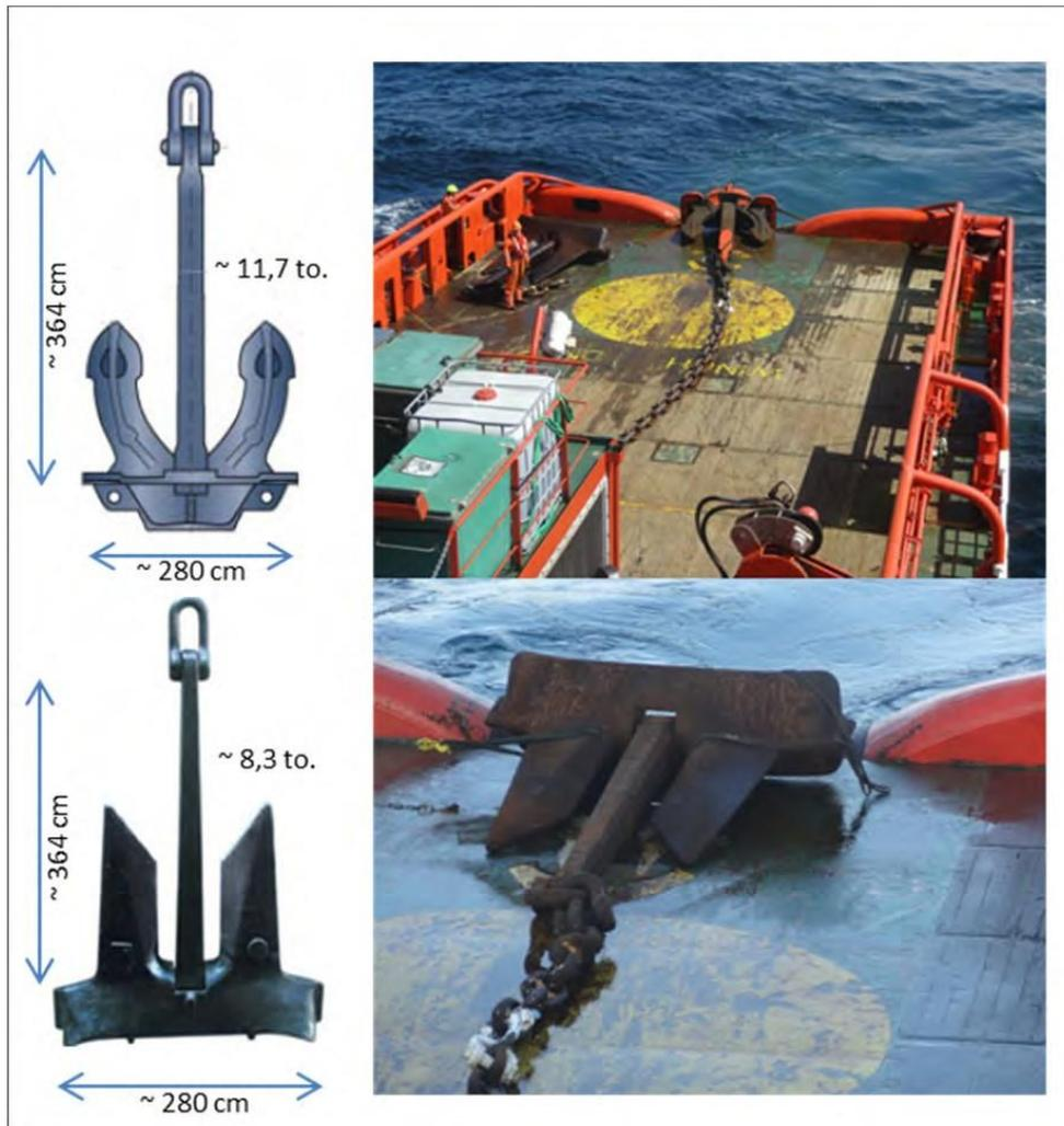
**Plate 6: Test anchors used: above: Hall – Anchor, below: HHP AC14 – Anchor**
