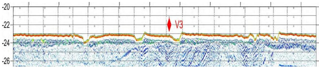
**Plate 7: SES profile line with anchor drop position[s] marked [V3]**
