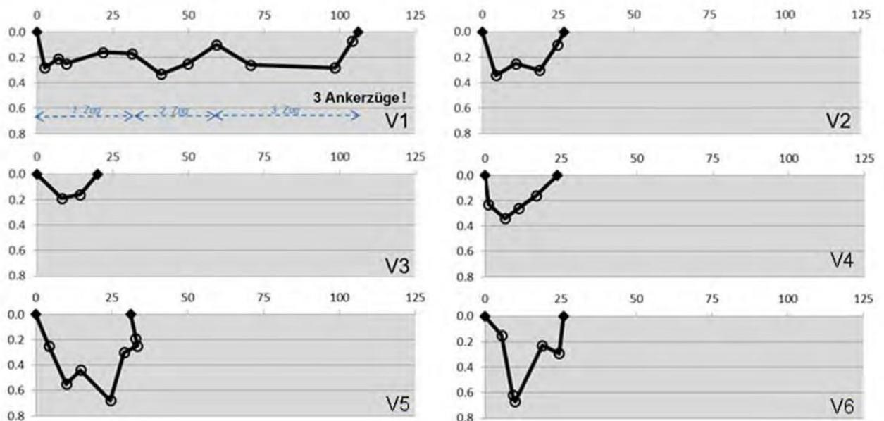
**Plate 16: Summary of all anchor tracks [depth profile] in test area VTG**
